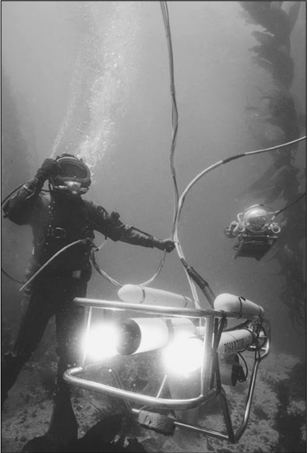
Remotely Operated Vehicles commonly accompany divers on many jobs today. The ROV can provide lighting and carry heavy tools for the diver.
